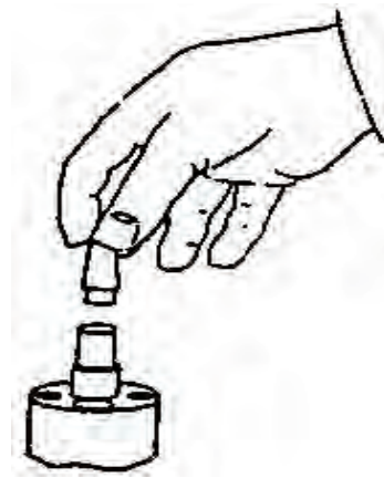
Fig. 8: Placing the Shank of the Dilator into the Inner Tube
