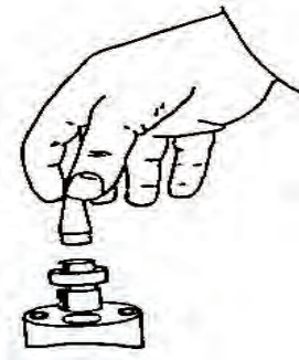
Fig. 9: Removing the Guide and Dilator
