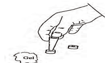
Fig.7: Placing the Top of the Dilator into the Inner Lumen
